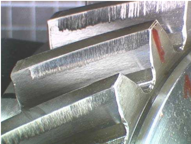
Fig. 2 Scuffing at the tips of helical gear teeth. Photograph courtesy of design unit, Newcastle University
