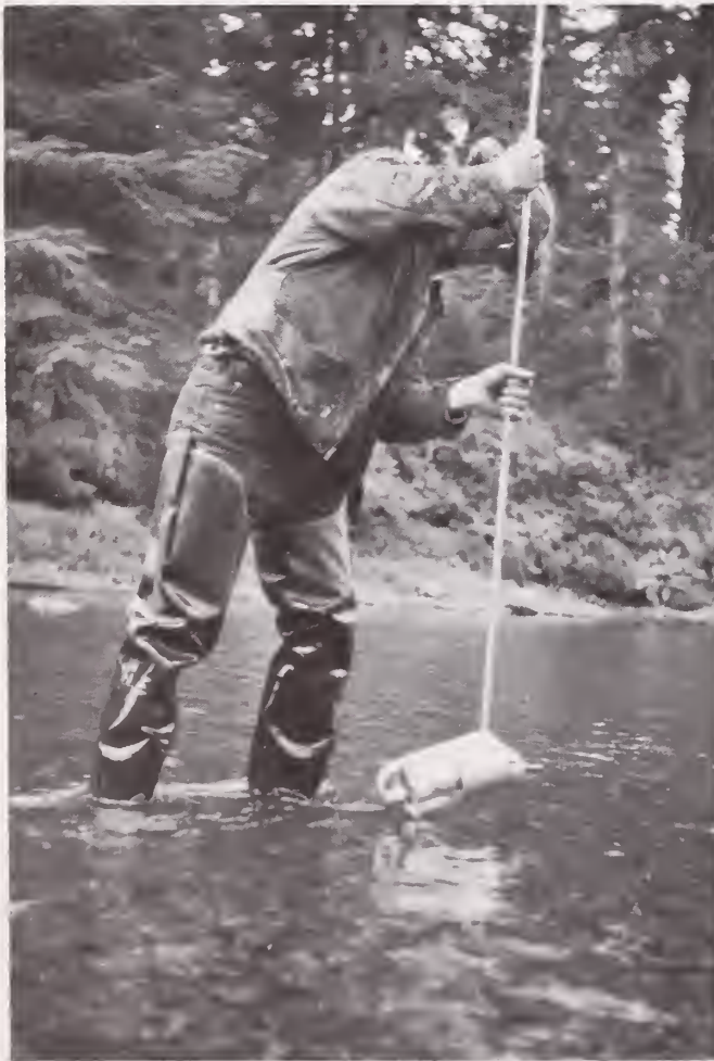
Figure 6 — Sampling suspended sediment with a USDH 48 sampler.
