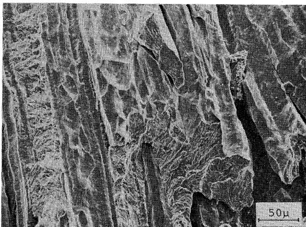
Photo. 14 Cracked surface occurred in electron beam weld metal of SUJ2 bearing steel. thickness; 30 mm, welding condition; 150 kV, 40 mA, 1,000 mm/min
