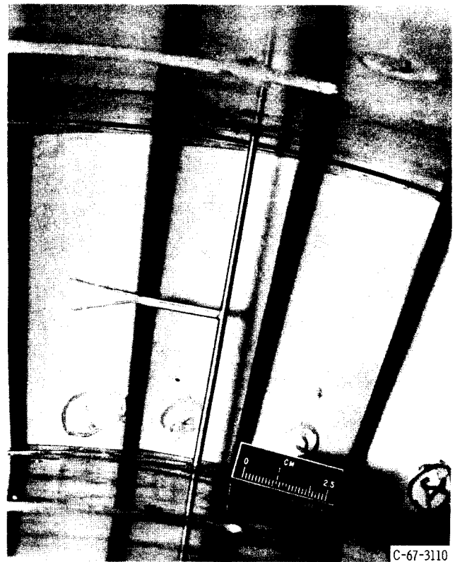
FIGURE 5. - PHOTOGRAPH OF A MODIFIED DESIGN PROBE INSTALLED IN TEST FACILITY.
