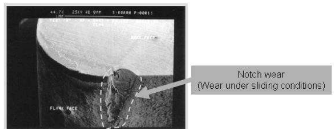
Figure 6. Notch wear observed on the flank face of an ISO K20 cemented carbide cutting tool after machining of Inconel 901 (Machado, 1990).
