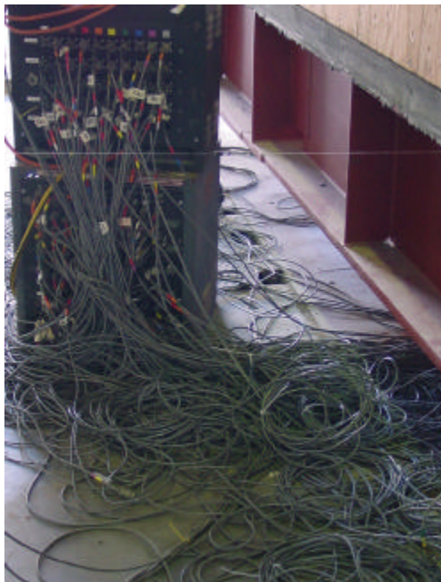
Figure 4. The real reason to go wireless! On the left is part of the traditional system wiring. Each mil-spec connector costs about $35, plus the soldering time and the $3000/channel Pacific Instruments amplifier at the end of each cable. Ms. Goethel's infrastructure is a lap-top computer and a Mote.
