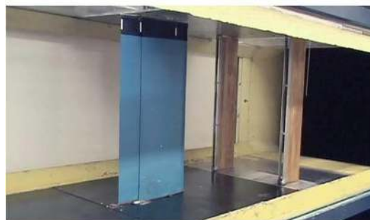
Figure 6: Photograph of the Experimental Model with Gust Generator in the Wind Tunnel Test
