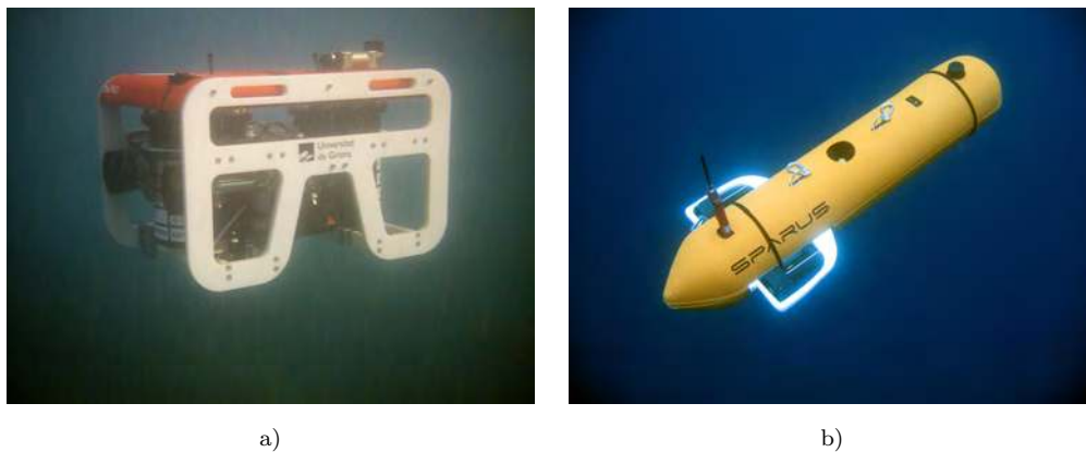
Figure 7.1: The AUVs from the University of Girona that were used for this research. a) The Ictineu AUV and b) the Sparus AUV.
