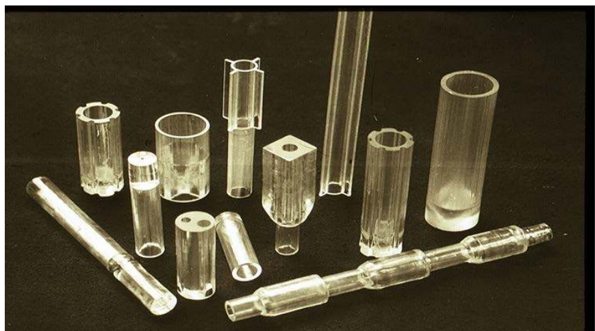
Figure 14. From [59] Monocrystalline sapphire profiles grown with TPS (technique of pulling from shaper) or VST (variable shaping technique) by the author of this paper with collaborators in the Solid State Physics Institute of Academy of Sciences of Russia.
