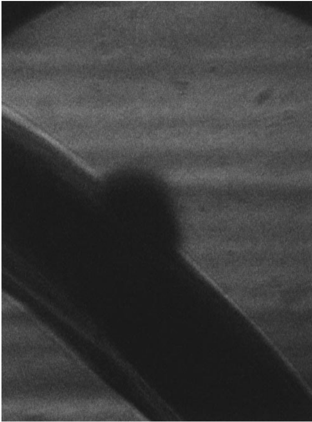
Figure 1 A hemispherical bubble trapped on a 500- \mu\text{m} wire in a sound field emits UV flashes of light and damages the metallic surface of the wire. It is not known whether this effect is caused by an imploding (hemispherical) shock, a jet, (Prosperetti 1997) or some other unidentified process.
