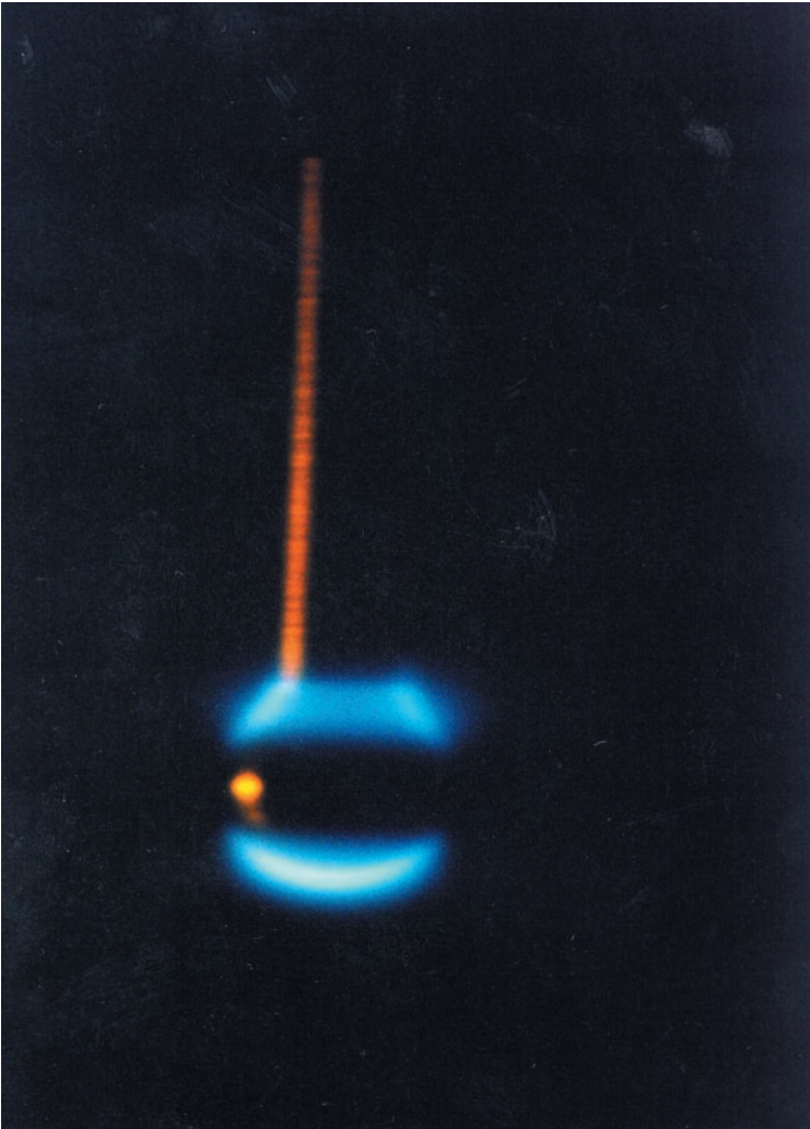
Figure 2 A metal sphere (4mm diameter) vibrating in water with a peak displacement of about 100\mu\text{m} creates a region of cavitation that transduces the sound into subnanosecond flashes of UV light. For this photo the light emission is enhanced by dissolving xenon into the water.
