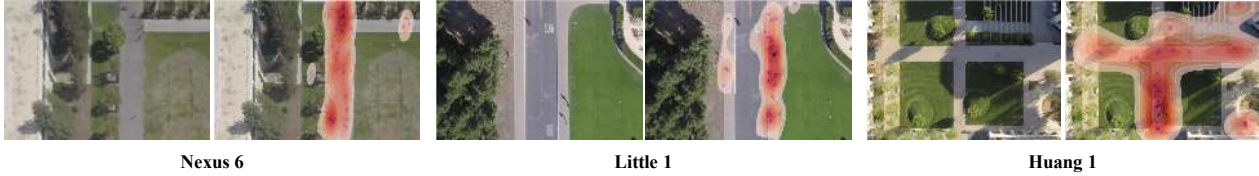
Figure 3. Using the generator to sample trajectories and the discriminator to validate those paths, we present highly accurate traversability maps for SDD scenes. Maps are presented in red, and generated only with 30 starting samples, illustrated as blue crosses.
