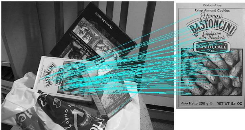
Figure 5.2: Example of the problem of object detection. Here, the box can be detected from the cluttered scene using the SIFT method from [207], where the blue lines indicate the matches with the training image.
