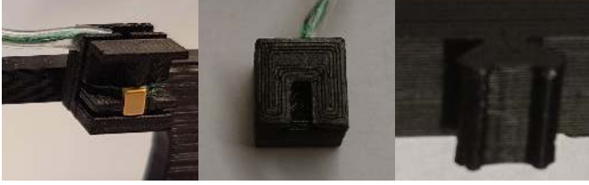
(a) Microphone in holder.(b) Microphone holder(c) AF microphone connector.
