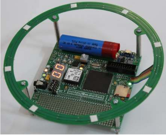
Fig. 2: The hardware of the designed sensor node. It is made up of a main processing board and a circular microphone array.
