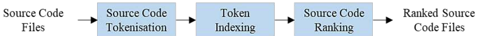
Fig. 5. IR-based technique works in three phases per original code. It accepts the code with their plagiarised and non-plagiarised code files as the inputs and returns plagiarism-suspected code files as the results.
