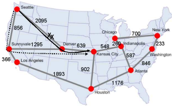
Figure 1: The Abilene backbone network. Numbers give the link weights, which are symmetric. The solid line between Seattle and Kansas City shows the lowest-cost route. The dotted line via Sunnyvale shows a deflected route, which avoids the Seattle-Denver link. The map and weights were taken from the Abilene Observatory ( http://abilene.internet2.edu/observatory/ ) on Dec 5, 2005.
