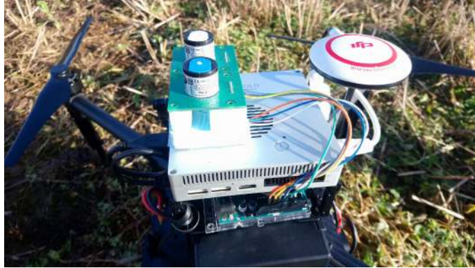
Figure 4: PID gas sensors connected to an Arduino Uno on-board the UAV.
