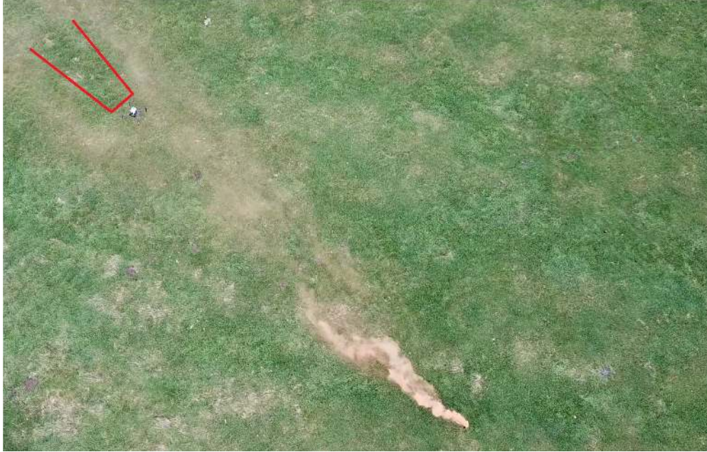
Figure 14: Visualisation of the UAVs effect on the gas dispersion using coloured smoke. A gap in the plume can be seen directly downwind of the platform, highlighted by the red lines.
