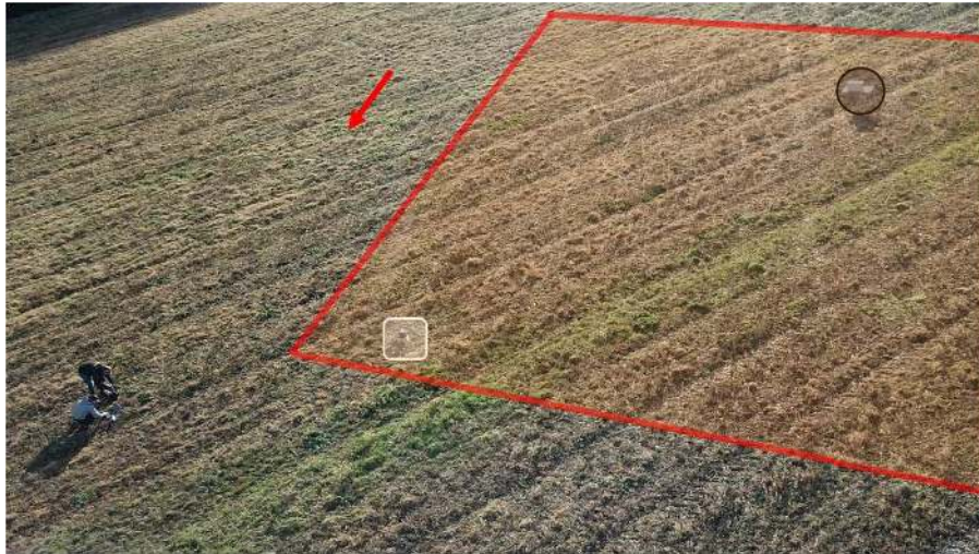
Figure 7: An example photo of the environment set-up for the experimental trials. The UAV begins the search at the white square and perform a sweep search pattern within the red area, which represents the prior distribution for the location of the diffusive source. The true position of the source is indicated by the black circle and the wind direction is implied by the red arrow.
