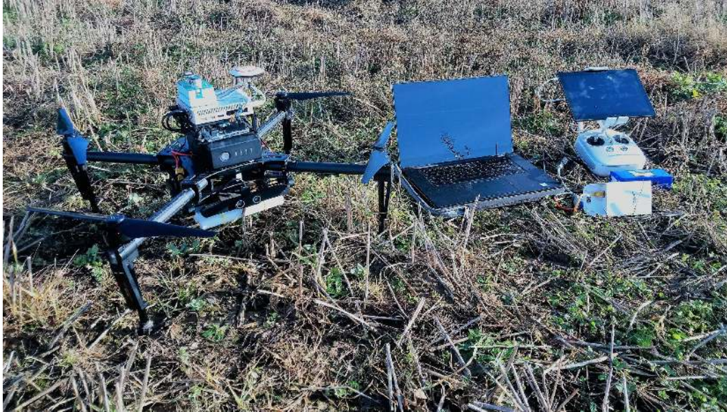
Figure 3: System components: DJI Matrice 100 UAV, ground station laptop, WiFi equipment and radio transmitter.
