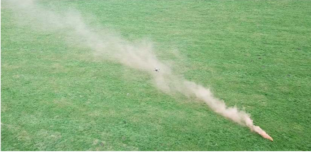
Figure 1: Visualisation of a UAV flying in the plume of a point source of emissions.
