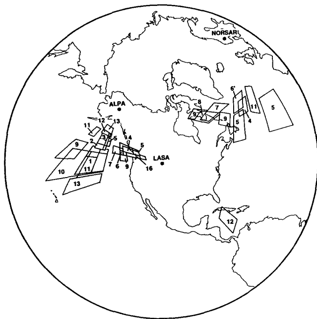
Figure 6. Map showing the positions of secondary microseism sources for storms in the north Pacific and Atlantic oceans, obtained by triangulation considering travel time differences. Position boundaries are drawn from the projection of half-power limits in the approach azimuth distribution determined for data from each array. The numbers refer to the sample sequence number for an interval spacing of 6 hr over the period 25 November 1973 to 29 November 1973.
