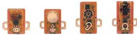
Cricket Sensors: Light sensor, touch sensor, sound sensor, resistance sensor.
