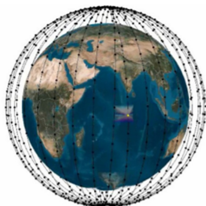
Figure 2. Constellation pattern of OneWeb system: 648 satellites distributed across 12 circular orbital planes at an altitude of 1200 Km; each plane inclined at 87°.
