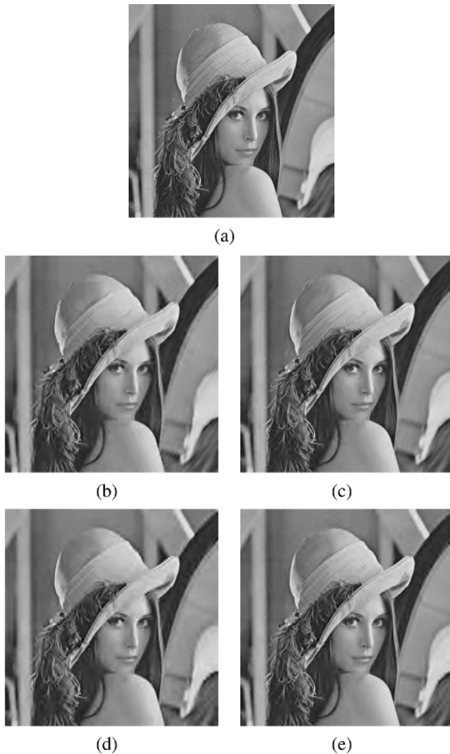
Fig. 13. Compression of Lena. (a) The original image. (b), (c) The image is compressed using the adaptive SFQ with directionlets at the bit rates 0.10 bpp (with the compression ratio 1:80) and 0.15 bpp (1:53), respectively. The numerical quality of the reconstructions is 30.92 and 32.56 dB. (d), (e) The image is compressed using the standard SFQ at the same bit rates. The quality is lower and is equal to 30.17 and 32.09 dB, respectively. The visual quality is also improved because the artifacts are oriented along locally dominant directions and are, thus, less annoying.
