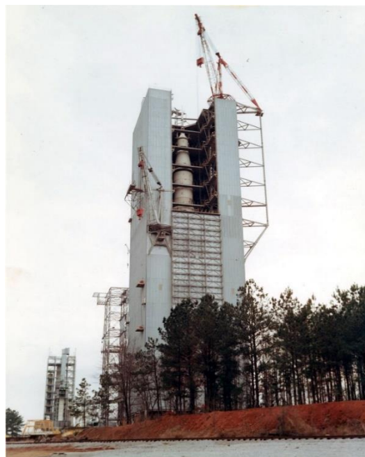
Figure 2. MSFC Advanced Saturn Dynamic Test Facility (Test Stand 4550) With Apollo SA-500D Installed.
