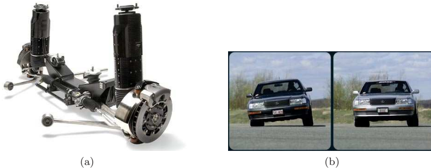
Figure 1.4: Electromagnetic suspension system by Bose Corp [17]. A front suspension unit is shown in (a), where (b) shows the body roll of the test vehicle in a aggressive turn, where the left picture is without and the right picture is with the Bose suspension system.
