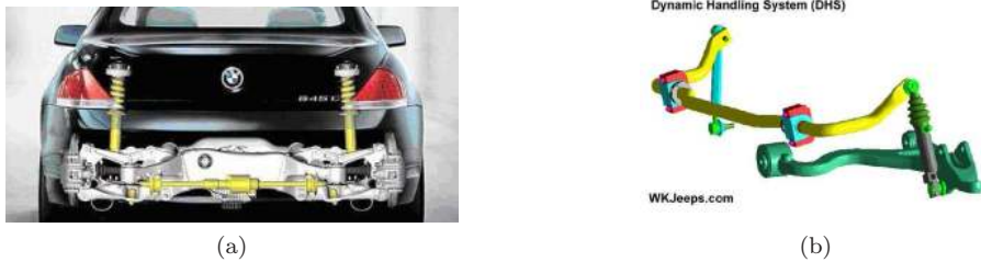
Figure 1.1: Commercial active anti-roll bar control systems. A rotary equivalent with the actuator situated in the middle [6] is shown in (a), where (b) shows the linear variant [7] with the actuator situated on the right in the picture.
