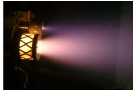
Fig. 11. Busek BIT-3 iodine thruster, from Ref. [83]
