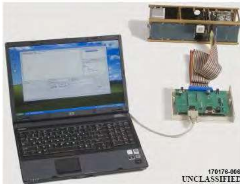
Figure 28. Electrical Ground Support Equipment (From Riot et al., 2011b, p. 6)
