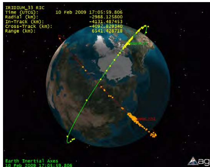
Figure 6. View of Iridium 33 and Cosmos 2251 orbits and debris 10 minutes post-collision (From Kelso, 2009)
