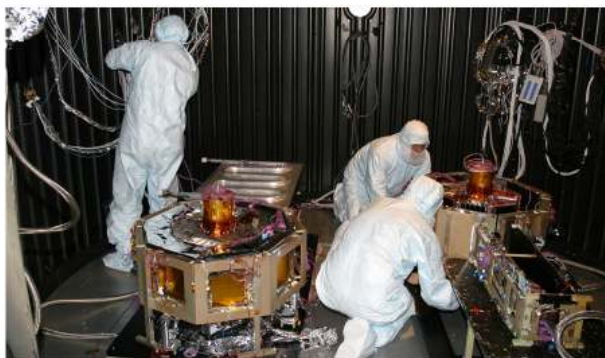
Spacecraft 2 and 3 in Thermal Vacuum Chamber
