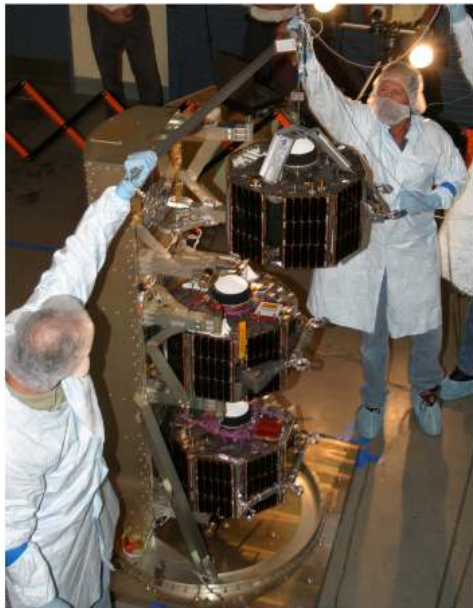
Test deployment of flight spacecraft from Pegasus Support Structure
