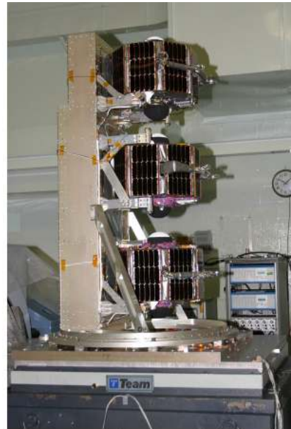
Pegasus Support Structure and Spacecraft Vibration Testing
