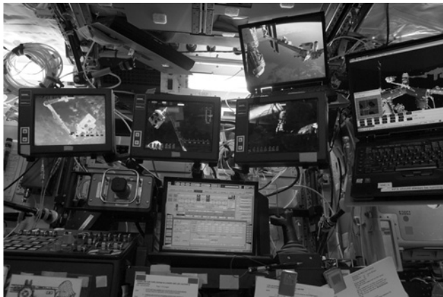
Figure 1.3. The robotic workstation is used by astronauts inside the Space Station to remotely operate the Space Station Remote Manipulator System. Source: National Aeronautics and Space Administration (ISS020-E-041812).
