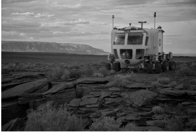
Figure 1.19. The Space Exploration Vehicle is a prototype pressurized crew rover. Source: National Aeronautics and Space Administration.
