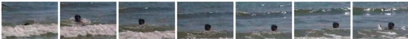
Fig. 16. Stabilization example. The top row shows a stabilized video sequence (courtesy of Matsushita [23]) of size 240 \times 352 \times 91 with 466,501 missing pixels. Each frame was transformed to cancel the camera motion and, as a result, parts of each frame are missing (shown here in red). Traditionally, the video would be cropped to avoid these areas and to keep only the region that is visible throughout. Here, the missing parts are filled up using our method to create video with the full spatial extent. The results here are comparable with those in [23].
