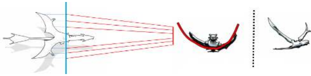
Figure 12: Both the body line and the DLOA at time t are projected onto a plane located at the root of the body part. For sketching secondary lines such as the wings, the character's main line (e.g. the spine) remains in a fixed reference pose. Last image on the right is the pose at the time of the sketched DLOA key frame.
