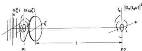
Fig. 11. When only the output intensity is of interest, the input, line spread function mask, and spherical lens may all be placed in the same plane for the OSD processor.
