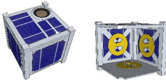
Figure 12: A spacecraft/rover hybrid is a planetary mobility platform sealed in one enclosure and actuated through three mutually orthogonal flywheels (for clarity, internal payload is not shown). By spinning the flywheels, one gives rise to surface reaction forces that make the rover tumble or hop. External spikes/feet (not shown here for clarity) are added to protect instruments and solar panels, and to improve traction. Trade-offs for spike design are discussed in Section 3.3.
