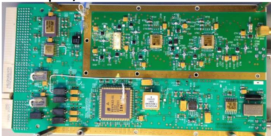
Example I/O Card: GPS RF
