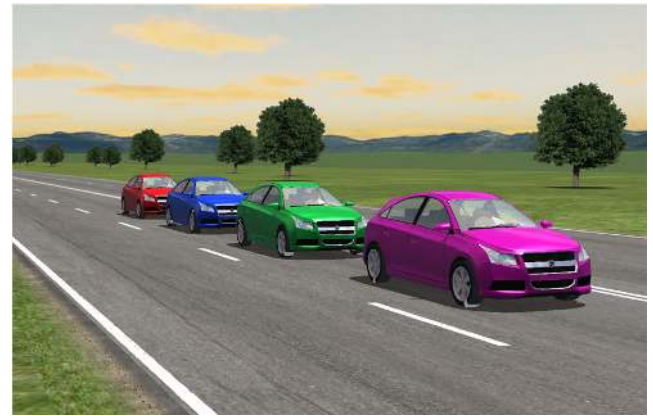
FIGURE 5. ACC platoon model established in CarSim.
