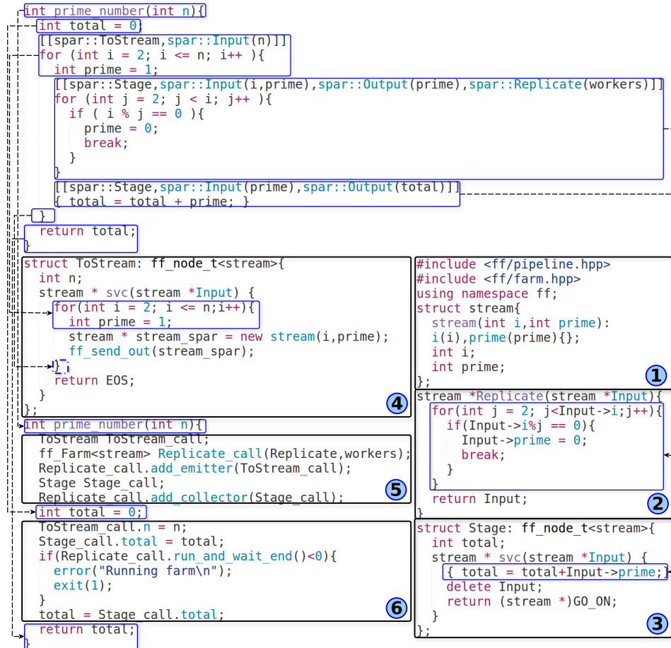
Fig. 3: Mapping the transformations to FastFlow generated code.
