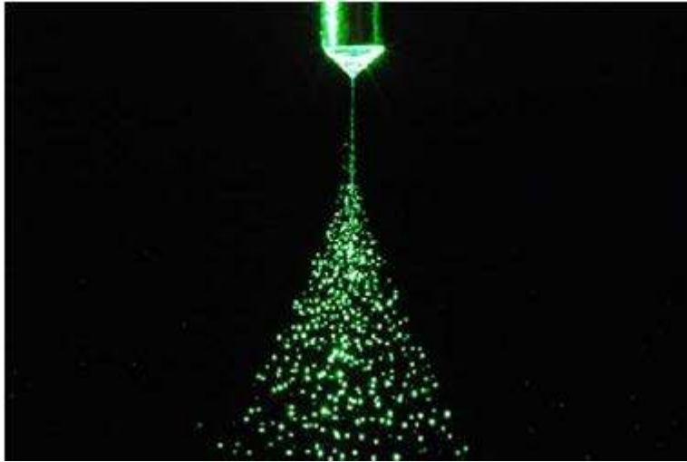
Figure 8. electro spray at the cone-jet mode. [19]
