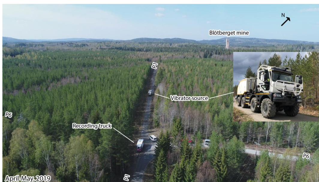
180 Figure 3. Field photos from the 3D seismic survey (April-May 2019) in the Blötberget mine. The survey was conducted using the 32t vibrator of TU Bergakademie Freiberg, 1266 receivers of which 414 were cabled (part of P1 and entire P3). The cabled profiles were used for live data quality control and sweep parameter tests. Earlier reported 2D profiles (years 2015 and 2016) were also along P1. Photos by Alireza Malehmir.
