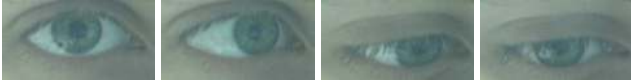
Figure 4. Typical training exemplars. These four images were captured during the calibration process for a gaze tracker. They were obtained by moving an animated spot to the four corners of the computer display (these are the first four milestones : see Fig. 3).
