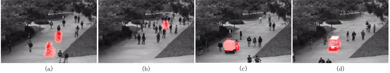
Figure 5. Examples of local abnormal event detections for UCSD Ped1 datasets. The objects, such as biker, skater and vehicle are all well detected.
