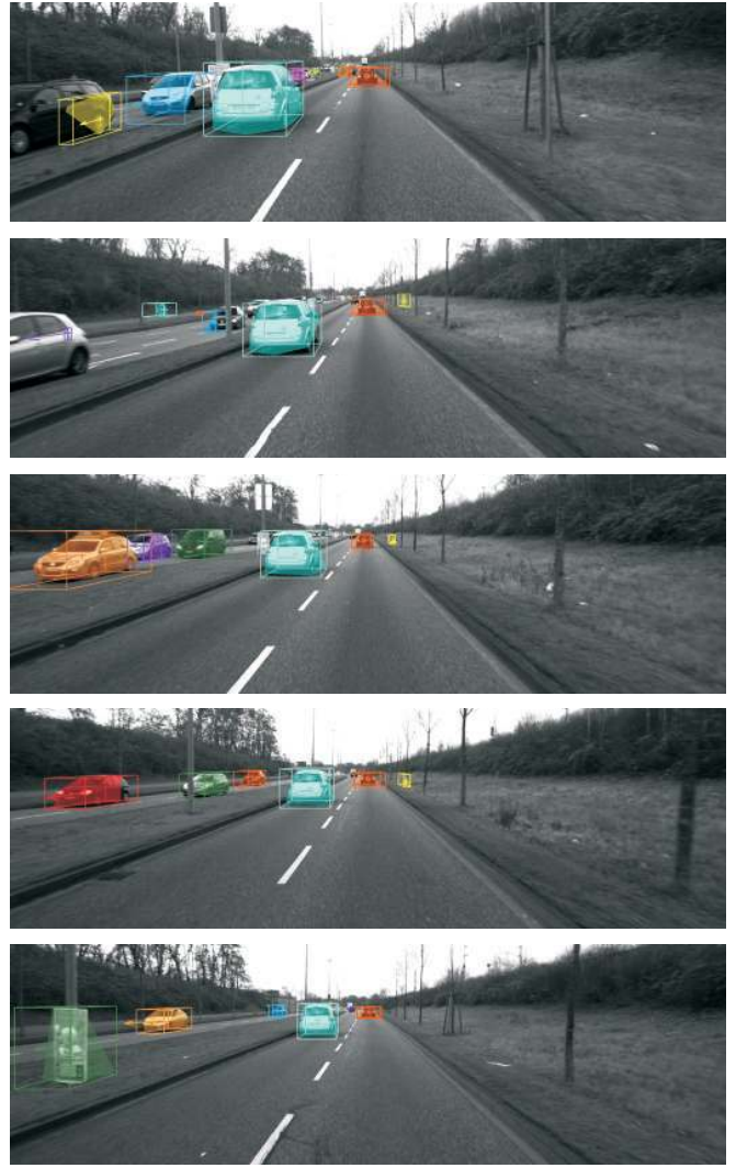
Fig. 7. Results on a rural road. The cars in front of the observer vehicle are tracked continuously within 15 s. The class-independent method detects the wheelchair user in the upper left area of the second frame. Static objects such as the advertisement or trees are detected as objects since egomotion is not compensated.
