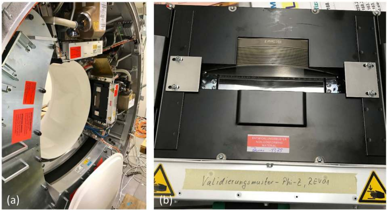
Figure 10: (a) The prototype of SparseCT with MSC installed and (b) a zoomed view of W4S16 MSC.
