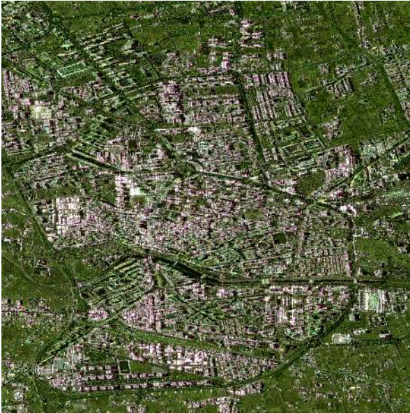
Fig. 4. Composite RGB image of the area under study in Murcia (Spain) formed by the average intensities. Channels: R = HH , G = VV , B = HH+VV
