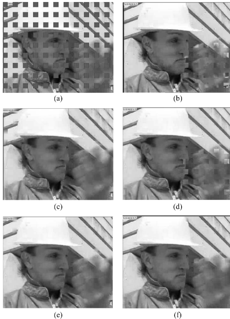
Fig. 9. Performance comparison of P-frame concealment results. (a) Error pattern (9.76 dB). (b) Zhang et al. 's algorithm (29.36 dB). (c) Lee et al. 's spatial method (29.48 dB). (d) Lee et al. 's temporal method (30.20 dB). (e) Lee et al. 's combined method (31.61 dB). (f) Proposed algorithm (32.23 dB).
