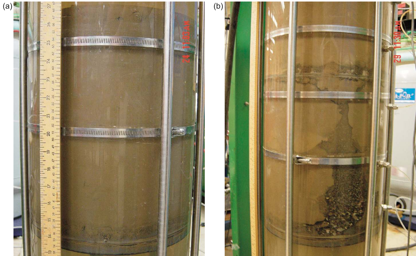
Fig. 13. Test specimen C-30-80-U: (a) before failure, i_{av} = 17 ; (b) after failure, i_{av} = 29 .
