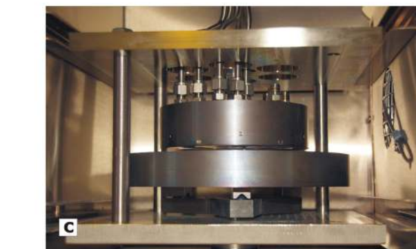
FIG. 9. (Color online) (a) Schematic of the bottom side of TNO's rotating spatial ALD reactor head, where the half-reaction zones are integrated into inlets surrounded by exhaust zones and gas bearing planes. (b) Schematic drawing and (c) photograph of the reactor. The reactor head and rotating substrate table with the substrate in between are placed in an oven. The substrate table is rotated by a servo-motor, connected by a drive shaft. The process- and waste gas lines are connected to the reactor head through an opening in the top of the oven.
