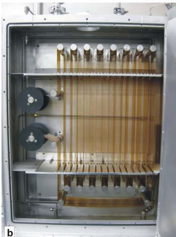
FIG. 3. (Color online) (a) Schematic drawing and (b) photograph of the Lotus Applied Technology spatial ALD reactor. The flexible substrate is woven back and forth between two precursor zones separated by an inert gas zone, in a serpentine configuration.
