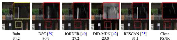
Figure 8. The difference maps (red boxes shown at the top-right) between the input rain image and results by deraining methods that suffer a PSNR drop. (Brighter indicates a higher difference.) We can see that [29, 40, 42, 25] tend to over-derain the image.
