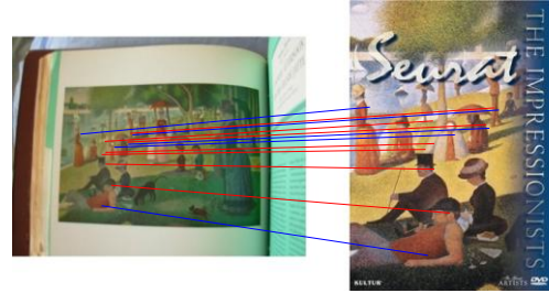
Figure 15. An instance of matching error due to SIFT drifting. Each line across two images denotes a match of two local features. The red lines denote the true matches that pass the spatial coding verification, while the blue lines denote those that fail to.
