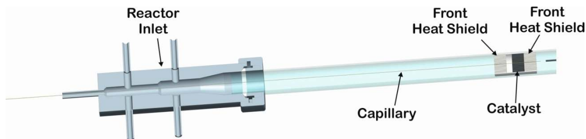
Figure 5. Scheme of the reactor setup with reactor inlet, capillary, front heat shield (FHS), catalyst (CAT), and back heat shield (BHS). The z -axis goes axially through the cylindrical quartz reactor, with z = 0 mm as the catalyst inlet and 10 mm as the catalyst outlet.
