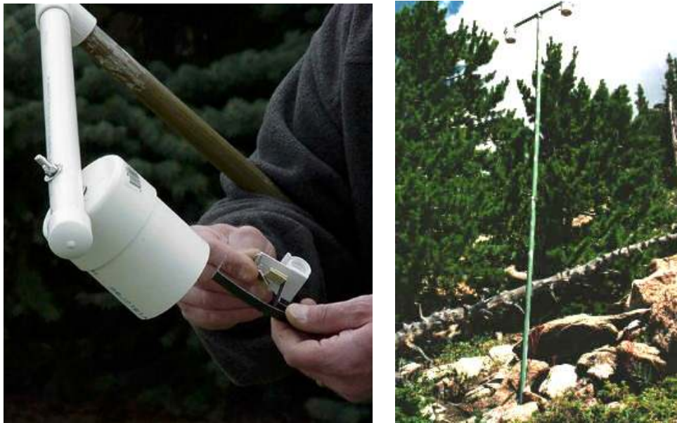
FIGURE 2. Pictures of the field equipment used with the passive sampler badges. Left: Rainshield and clip to hold badges. Right: sampling system pole with two rainshields in field use. The sampling systems are placed in clearings such as the rock field shown. The poles and the outside of the rainshields are painted to blend into the surroundings.
