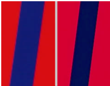
Figure 10 Image of red/blue slant edge used in computing the chrominance SFR for Canon 10 (left) and Sigma SD10 with Foveon X3 image sensor (right). The sharper edges in the Foveon X3 image are evident.
