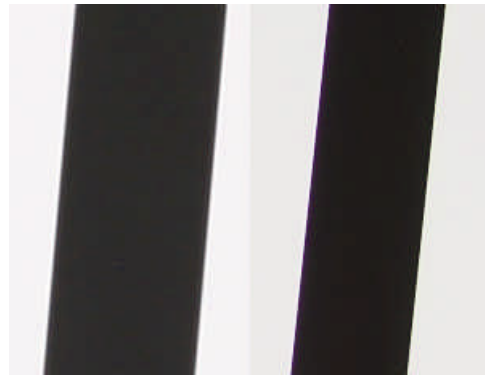
Figure 7 Images of slant edge used in computing the luminance SFR for Canon 10D (left) and Sigma SD10 with Foveon X3 image sensor (right). The sharper edges in the Foveon X3 image are evident.
