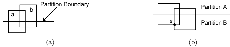
Fig. 14. (a) An intersection between objects a and b is reported from both partitions into which they are inserted, creating a duplicate result. (b) The reference point method for online duplicate avoidance only reports an intersecting pair if a point in the intersecting region, x , is within the current partition. The point must be chosen consistently, such as always the lower left corner.
