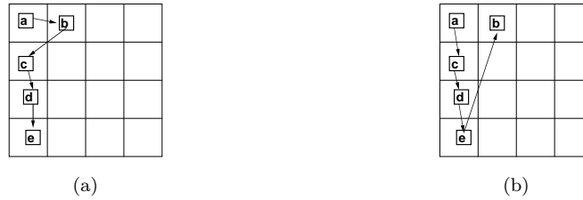
Fig. 22. (a) A linear order, where object a 's neighbors, b and c are nearby. (b) A linear order in which one of object a 's neighbors, c , is nearby, but the other neighbor, b , is not.
