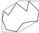
Fig. 35. An MBR approximation can be improved by adding two more sides, parallel to each other.
